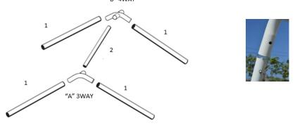
Starting at the front of the unit assemble the horizontal side framework to the prebuilt roof. Complete the assembly of one side before working on the other.
