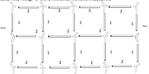
Step 2: Assemble roof framework
