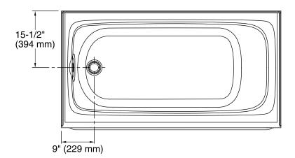
No change in measurements if connected with drain illustrated. (K-11677)
