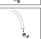
(8) Connect hot and cold inlet supply hoses to supply stops. For 1/2" connection; use 3/8" male to 1/2" female adapter for installation. Adapters are optional and not provided with the faucet.
