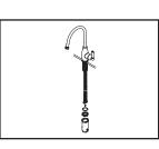
(6) With washer inside locknut, thread locknut onto faucet body from underneath of the sink. Tighten locknut with help.
