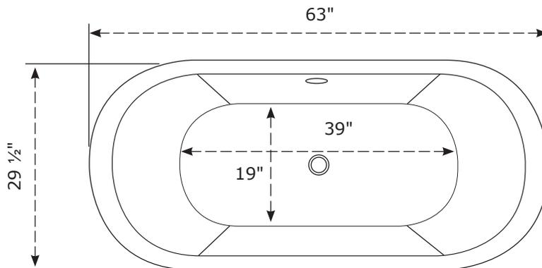
Vertical air jets can be installed on this bathtub. The blower must be installed in a remote location and not within the outer shell of the bathtub.
