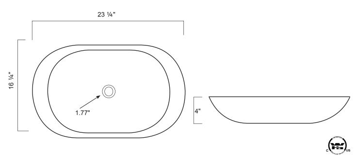
$\label{eq:Diagrams} \begin{array}{c} \text{Diagrams not to scale} \\ \text{All measurements} \pm 1/4 \text{"} \\ \text{1 year limited warranty against manufacturer's defects} \\ \text{This sink complies with CSA Standards} \end{array}$
