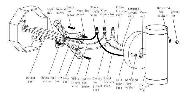
Details 1, 2, 3 show the proper procedure to secure wires with Wire Connectors.
