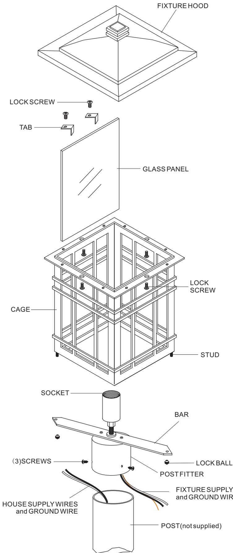
1. Before beginning the assembly/installation, carefully unpack and identify parts, referring to the illustration.
