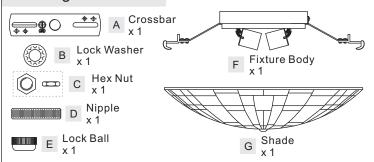
E. Place the Fixture Body (F) back over the Nipple (D) and secure with Lock Ball (E). Hand tighten until snug.
