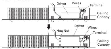
C. Connect the Live Wire from Driver to Port "L" on the Terminal, which is the corresponding port of the Live Wire from LED Panel. Connect the Natural Wire from Driver to Port "N" on the Terminal, which is the corresponding port of the Natural Wire from LED Panel.
