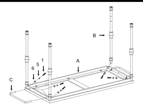
Note: Do not tighten bolts completely until step 3 is complete.
