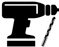
Drill and drill bits Perceuse et forets Taladro con brocas ø1/8" (3mm) & ø5/16" (8mm)
