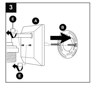
4. Attach mounting plate (B) to outlet box (not included) using existing washers and outlet box screws or the machine screws (BB). NOTE: If the outlet box screws required for your outlet box are of a different size than the machine screws (BB), consult a licensed electrician before proceeding.
