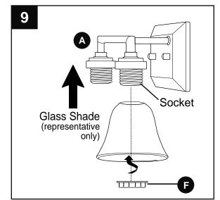
Install standard-base bulb(s) (not included). Use 60-watt max. incandescent bulb(s) or CFL/LED equivalent.
