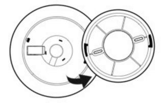
Remove cap to expose screw base.
