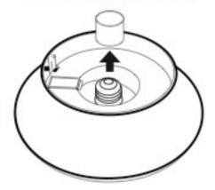
3 Screw LED fixture into socket just like a light bulb.
