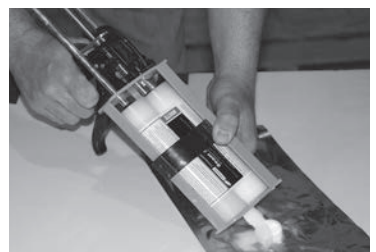
FIGURE 13: LEVELING THE PLUNGERS
