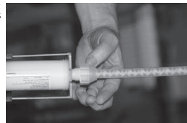
FIGURE 14: ATTACH STATIC MIXING TIP
