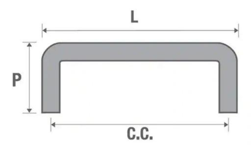
C.C = Center to Center (Distance between the drill holes)
