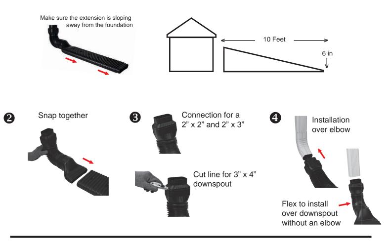
The purpose of downspout extensions is to move the high volume of rainwater from the roof and direct it away from the foundation. Any water that may seep from the connections will be less than the amount of water actually saturating the surrounding ground from the rainfall.
